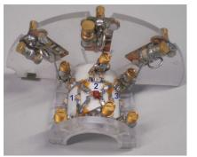
Fig. 2: 3-Channel receive array. The balun in the input circuit is mounted on the vertical plate.
