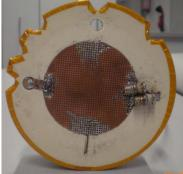
Fig.1: Capacitive tunable linear patch antenna. The slots along the edges are provided for cable routing.
